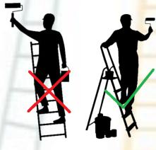
Always maintain three points of contact when climbing up and down or performing work from a ladder.
