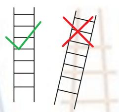
Make sure your ladder is placed on level, stable ground. Never climb a ladder unless all the feet are in contact with the ground.
